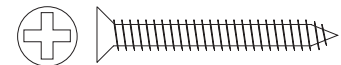
1 1/4" Phillips Flat Head #8 Screw (2) Brass - Packaged Separately with Pipe Holder and Standoff.
